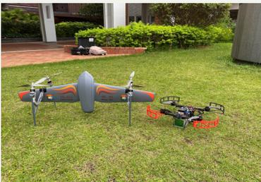
(Dr Zhang's latest projects: Left: energy saving UAVs; Right: efficient and accurate 3D reconstruction based on LiDARs.
